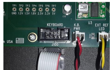
Figure 4-2 Boot-Loader jumper location
