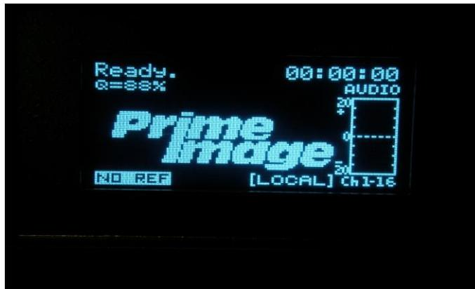
If a Genlock signal is not present, the TT3500AP will either Free-Run or “Lock to Input” depending on the menu selection for “NonGenlock Mode” found under the SYSTEM menu.
