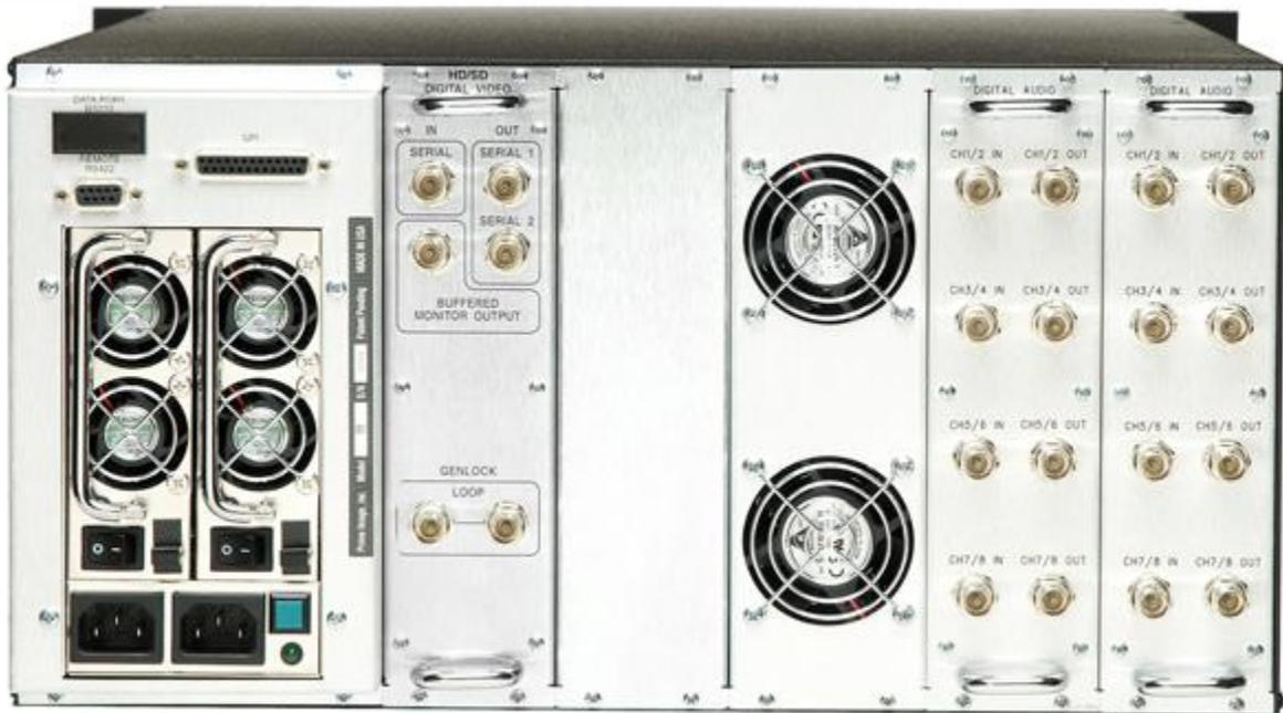
*Figure 3-1. Rear Panel Connectors*
